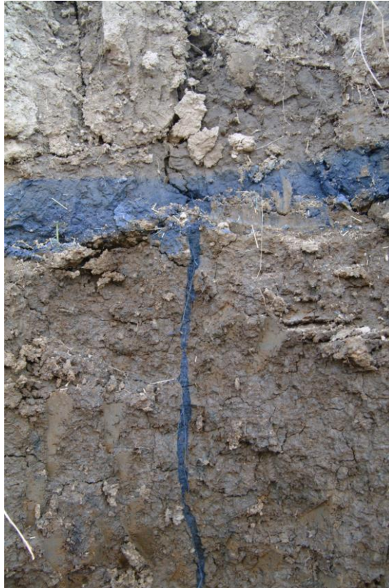
Figure 9.9. Route of water in clayey soil traced using methylene blue dye. Photo: Visa Nuutinen.
