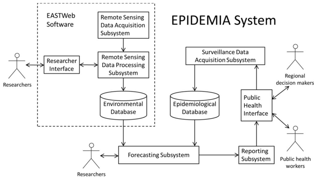
**Figure 2:** Block diagram depicting the major subsystems and users of the EPIDEMIA system
