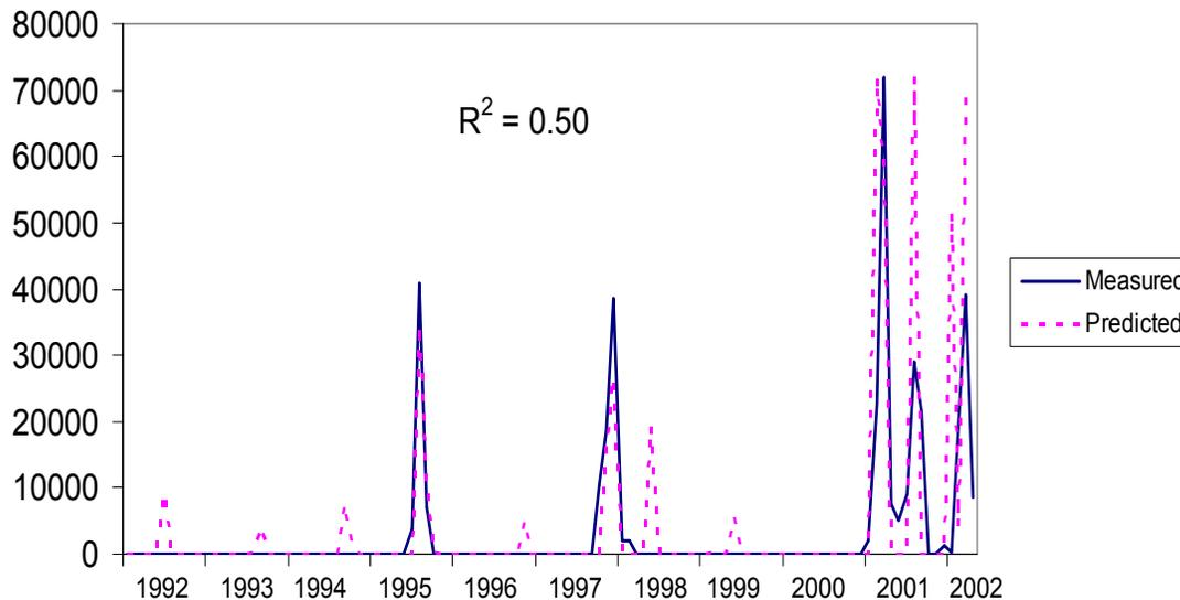
**Figure 3 Results of 1 month ahead forecast of Dam Spillage using dataset from Ahning Dam.**
