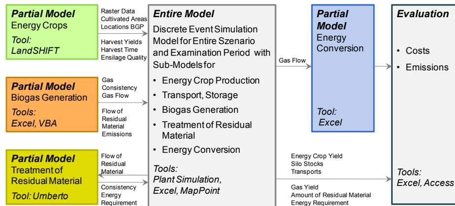
Figure 1. Model pipeline of biomass conversion
