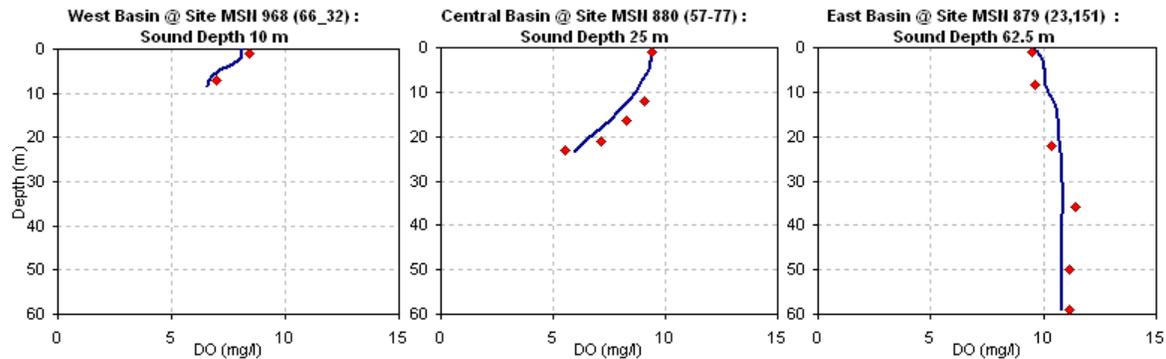
**Figure 5.** Comparison of measured versus calculated dissolved oxygen profiles for selected sites in the west, central and east basin of Lake Erie for the 1994 simulation after 80 days of simulation on July 28<sup>th</sup>
