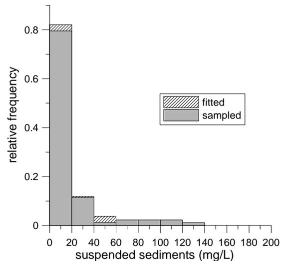
**Figure 6.** Histogram of sampled suspended sediment concentrations at Bad Kösen fitted with a gamma probability distribution.
