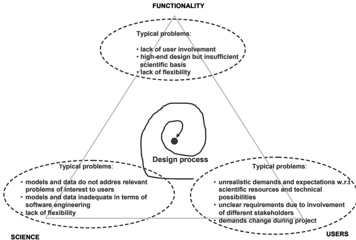
Figure 1. Iterative design of a DSS with typical problems that arise if one of the aspects of the design is overemphasized.
